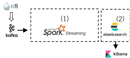
Figure 5. Proposed Kappa Architecture
