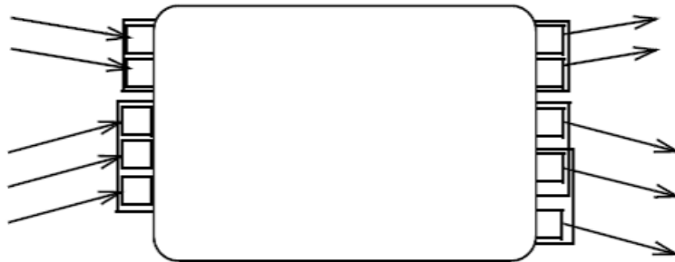
Figure 16.23 Alternative input/outputs using ParameterSet notation
