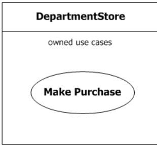
Figure 18.9 Notation for UseCase owned by Classifier
