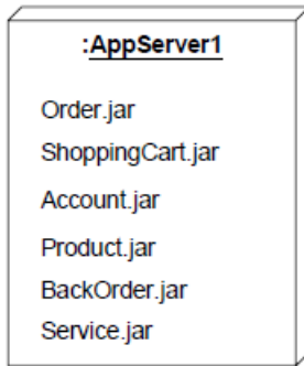
Figure 19.4 Textual list based representation of DeployedArtifacts.
