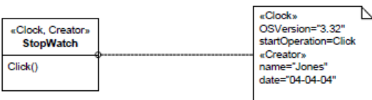
Figure 12.30 Using Stereotypes and Showing Values
