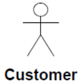
Figure 18.6 Actor notation using stick-man
